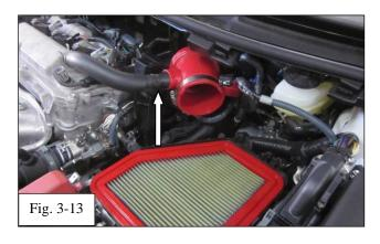
(m) Install the crankcase vent to the TRD coupler and secure it with the spring clamp (Fig 3-13).
