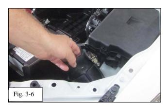
(f) Lower the TRD air box inlet tube into position behind the driver side headlight as shown (Fig. 3-6).
