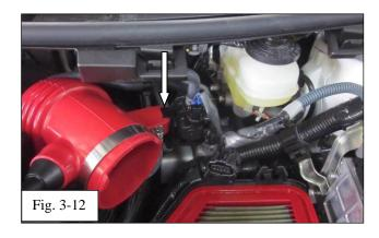
(l) Insert the VSV bracket into the slot in the TRD coupler (Fig. 3-12).
