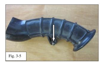
(e) On a table or bench away from the vehicle, install the spacer into the air horn until it is flush with the bottom of the boss (Fig. 3-5).
