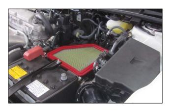
(j) Install the TRD air filter (Fig 3-10).
