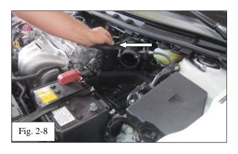
(h) Disconnect the crankcase vent hose from the air intake bellows (Fig. 2-8).
