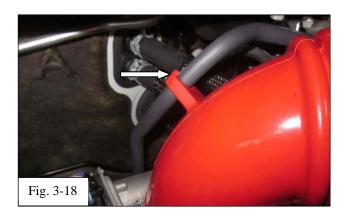
(r) Secure the vacuum hose using the clip on the back of the coupler (Fig. 3-18).
