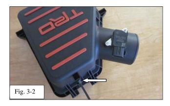
(b) On a table or bench away from the vehicle, install the tree mount zip tie to the rear of the air box (Fig. 3-2).
