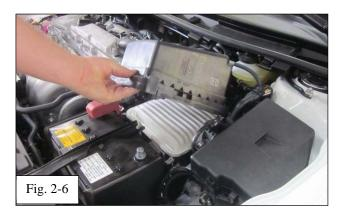
(f) Lift and remove the upper air box (Fig. 2-6).
