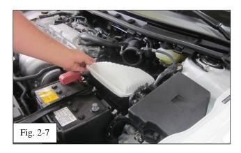
(g) Remove the OEM air filter (Fig. 2-7).
