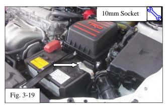
(s) Do a final check to ensure all wires and hoses are secure. Re-connect the negative battery cable to the negative battery terminal (Fig 3-19). Torque to 5.4 Nm (48 in-lbf).
