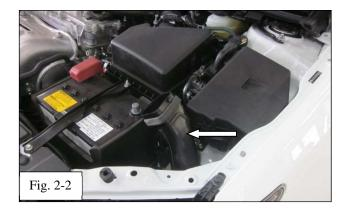
(b) Remove the OEM air box inlet tube (Fig. 2-2).
