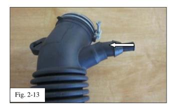
(m) On a table or bench away from the vehicle, remove the plastic PCV connector from the OEM coupler (Fig. 2-13).
