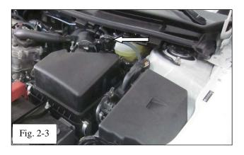
(c) Unplug the MAF sensor and unclip the wiring harness from the OEM air box lid (Fig. 2-3).
